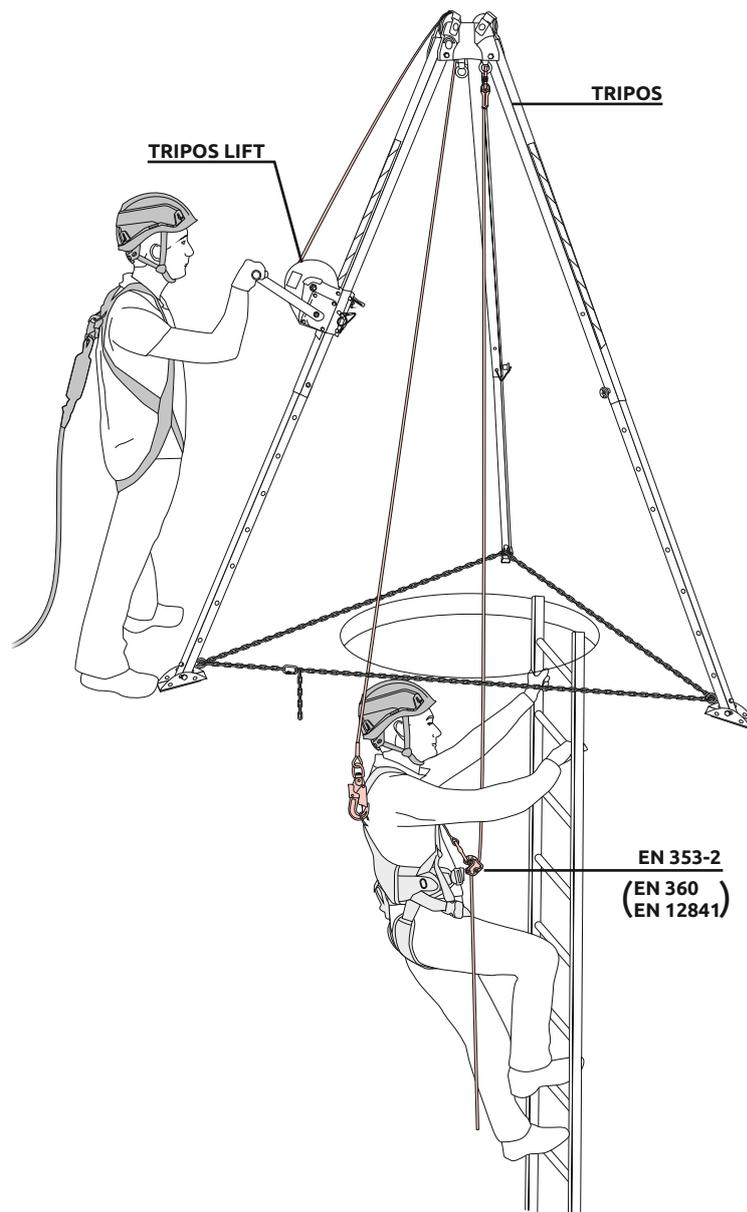
TRIPOS and two COBRA LIFT, two users, with risk of falling from a height
